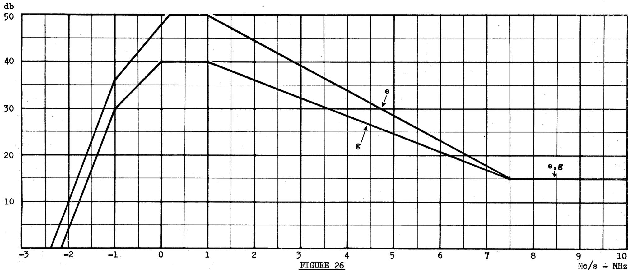
819-line system. Protection from CW or sound-signal interference
