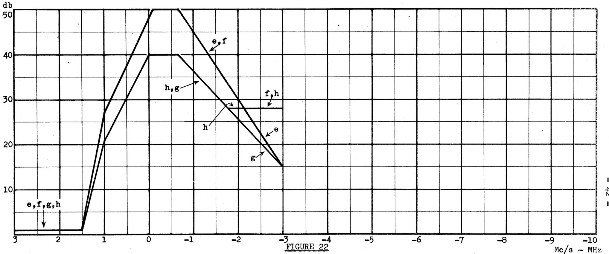
405-line system. Protection from CW or sound-level interference
