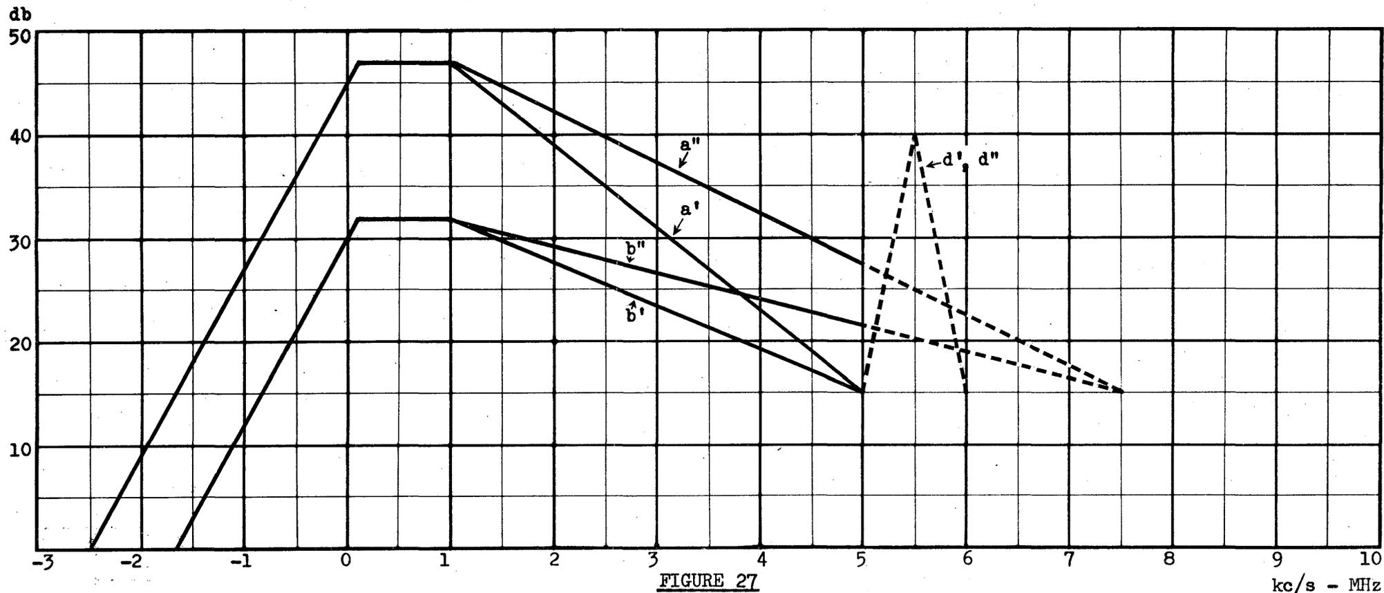
Belgian 625-line and 819-line systems. Protection from vision-signal interference
