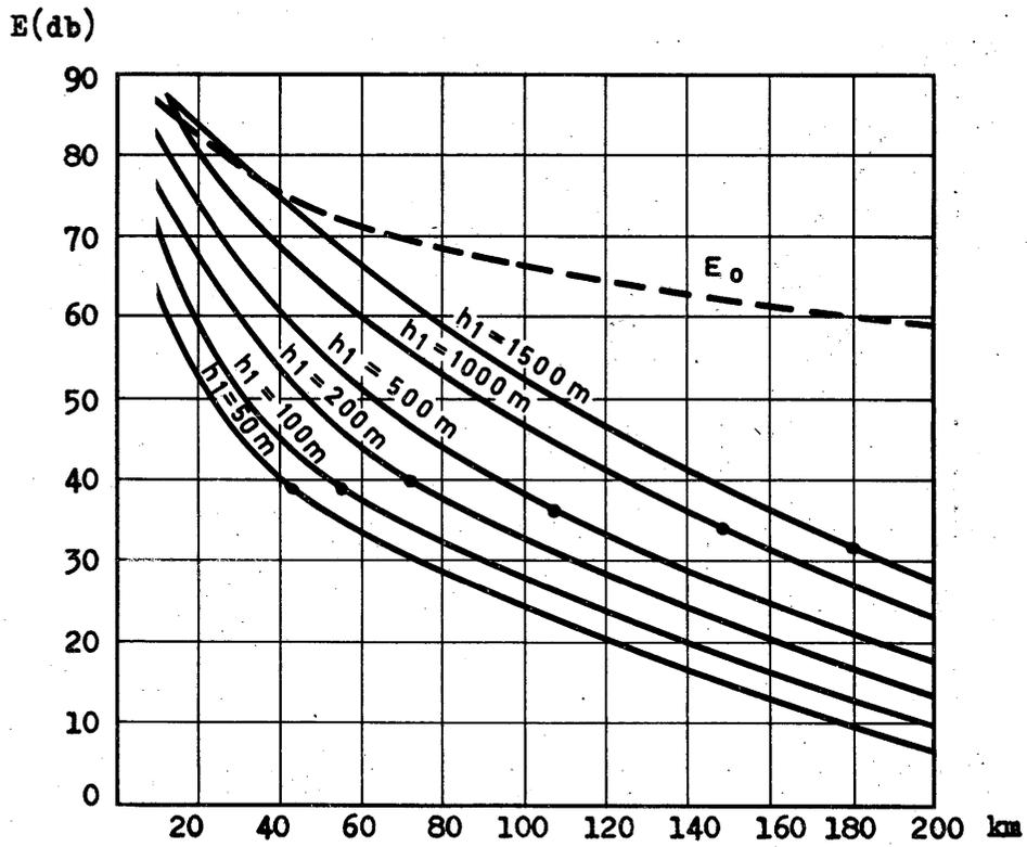
Half-wave dipole -  $h_2 = 10$  m
