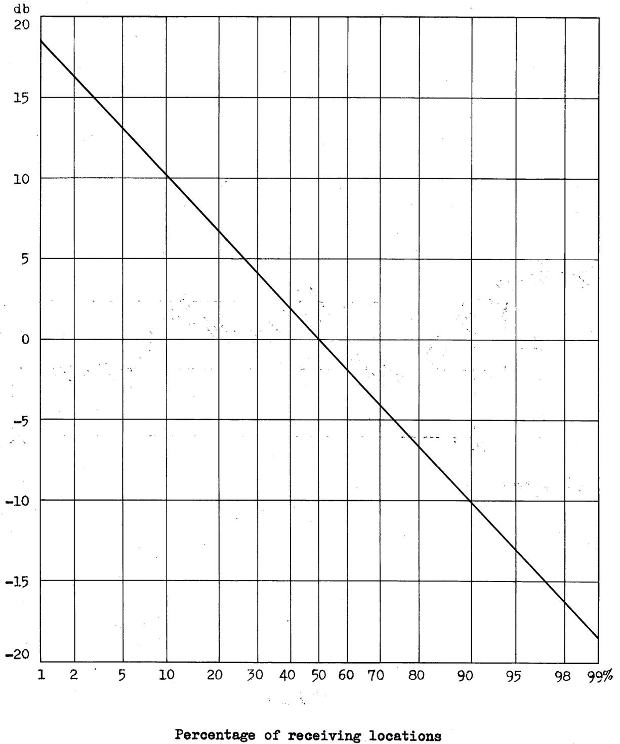
Ratio, in db, of the field strength for a given percentage of receiving locations, to the field strength for 50% of receiving locations
