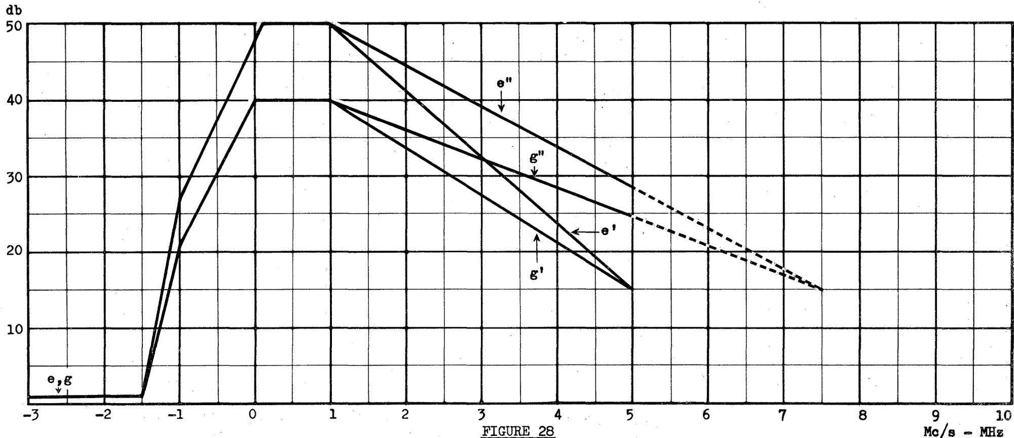
Belgian 625-line and 819-line systems. Protection from CW and sound-signal interference
