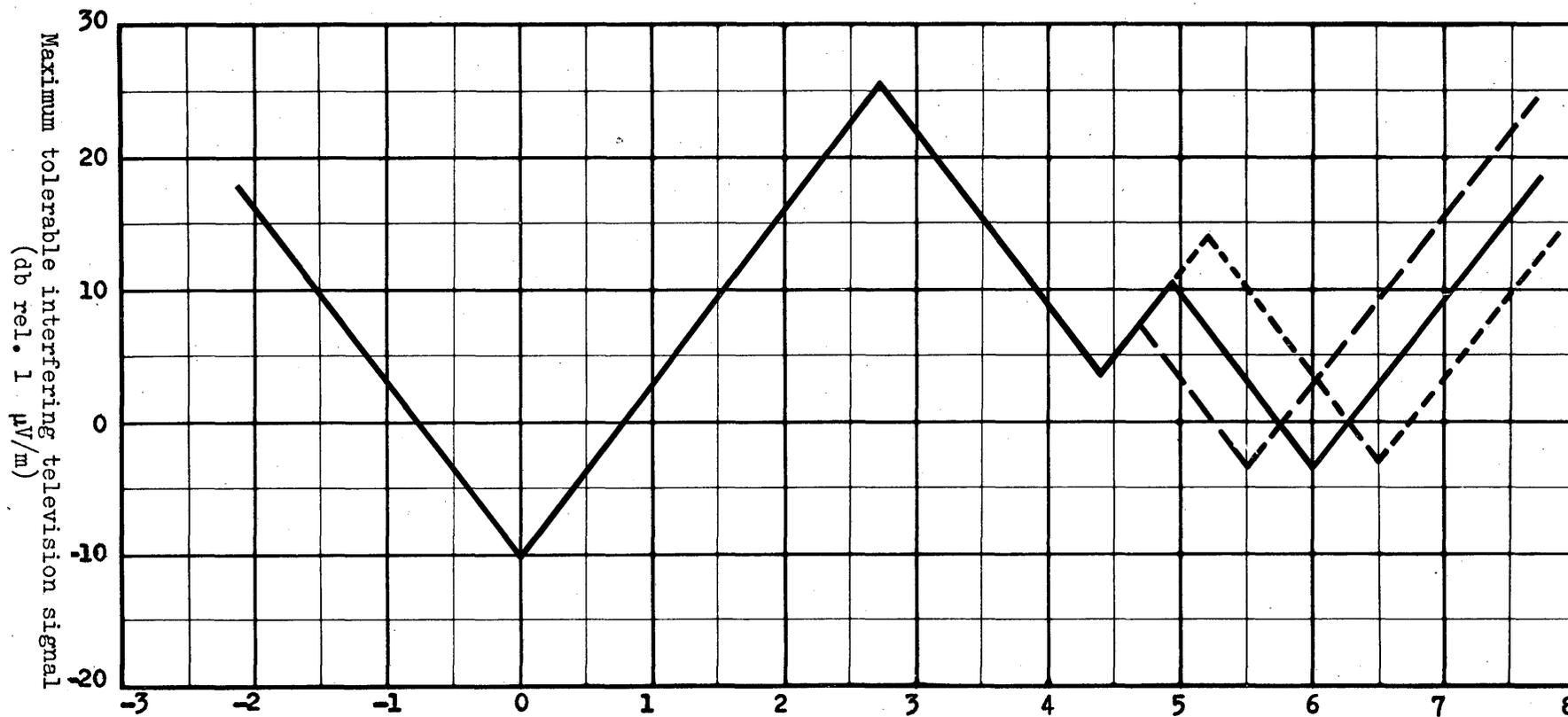
Centre frequency of pass-band of radionavigation receiver relative to the vision carrier frequency of the interfering television signal (Mc/s)
