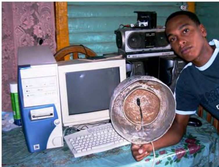
Picture N° 15: Antenna made of kitchen pots
