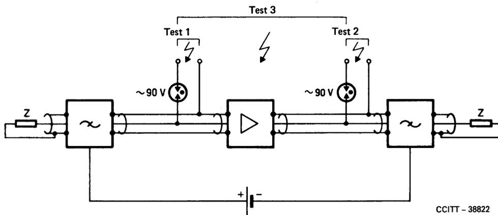
Note - The value of Z will be chosen in conformity with the system under test.
