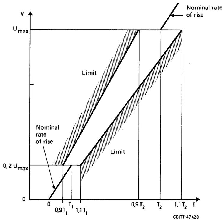
*Note* – Spark-over test waveform (nonconducting) must be within enclosed limits.
