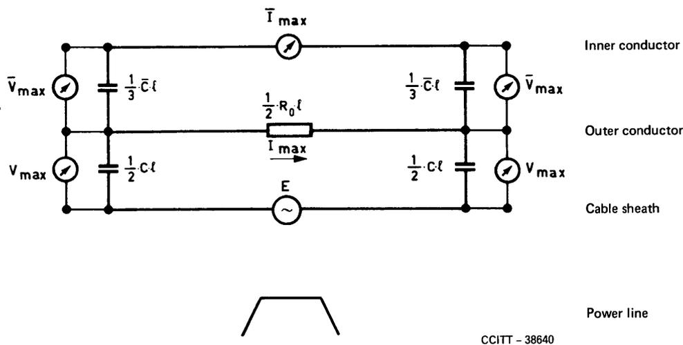
$E$  = longitudinal voltage induced in the cable (volts)
