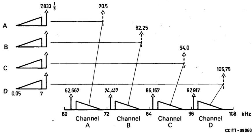
Note – The carrier frequencies are multiples of 11.75 kHz and can be derived from a common generator frequency:
