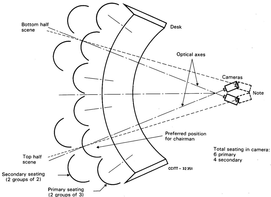
Note - Solid line cameras are for cross-fire. Dashed line cameras are for parallel-fire.
