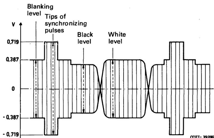
Note – The voltages shown are the values measured at a zero relative level point for television transmission in the 12 MHz system.
