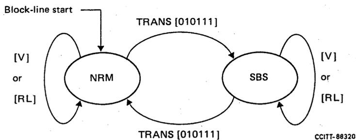
Note — The same motion vector coding method is applied for both NRM and SBS modes.
