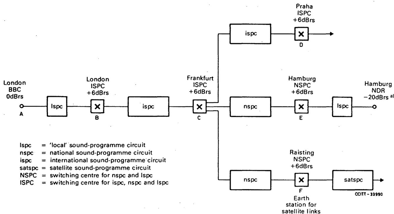
Note – Maximum level of sound programme signals: +9dBm0s (this means +9dBm at a 0dBrs relative level point and +15dBm at a +6dBrs relative level point respectively). The value of +9dBm corresponds to a peak voltage of 3.1 V which is the maximum value of a sine-wave signal of 2.2 V r.m.s.
