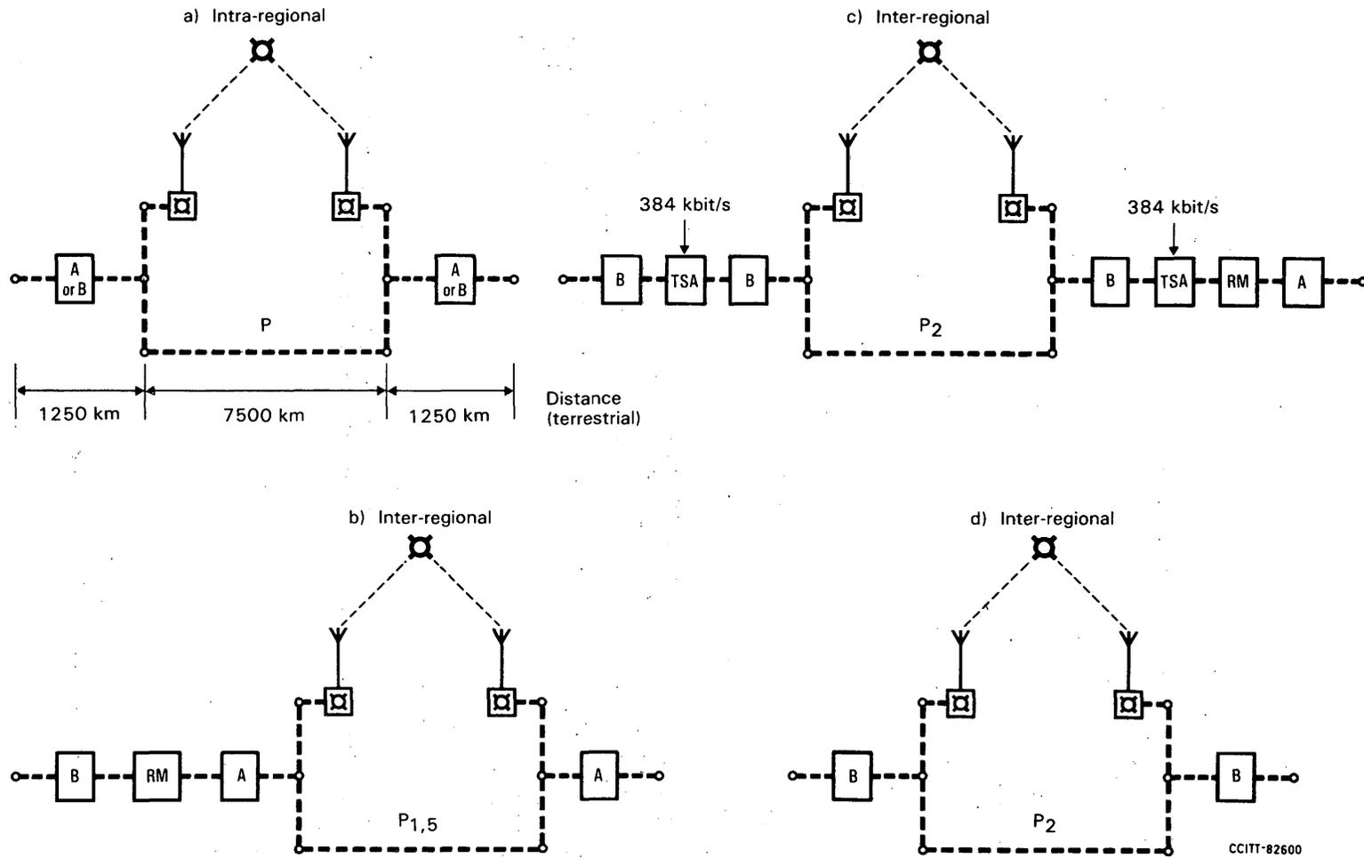
Note - The distances shown in Figure 2a/H.110 are applicable to Figures 2b/H.110, 2c/H.110 and 2d/H.110. These distances refer to terrestrial transmission. Equivalent distances relating to satellite transmissions are for further study.
