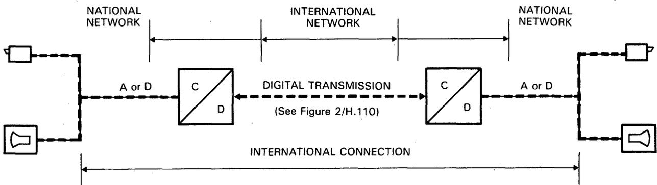
A or D – Wideband analogue or digital transmission or both all providing equivalent quality.
