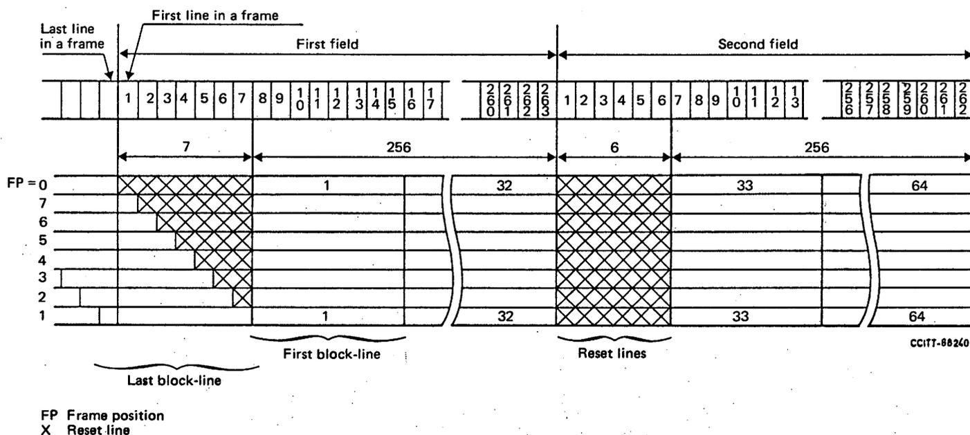
*Note* — When the last line in a frame falls on the  $n$ th line of the last block-line,  $FP = \text{mod}(n, 8)$ .
