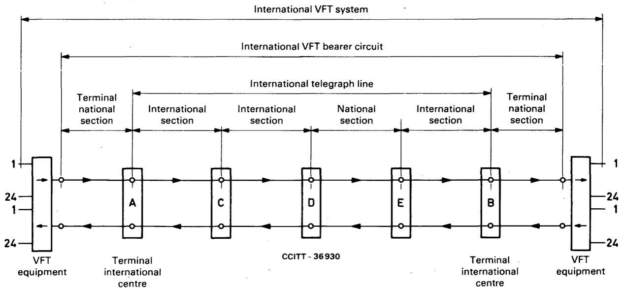
Note — At the intermediate centres C, D and E and at the terminal international centres A and B, the signals transmitted are at audio frequencies. At these points it is possible to make measurements.
