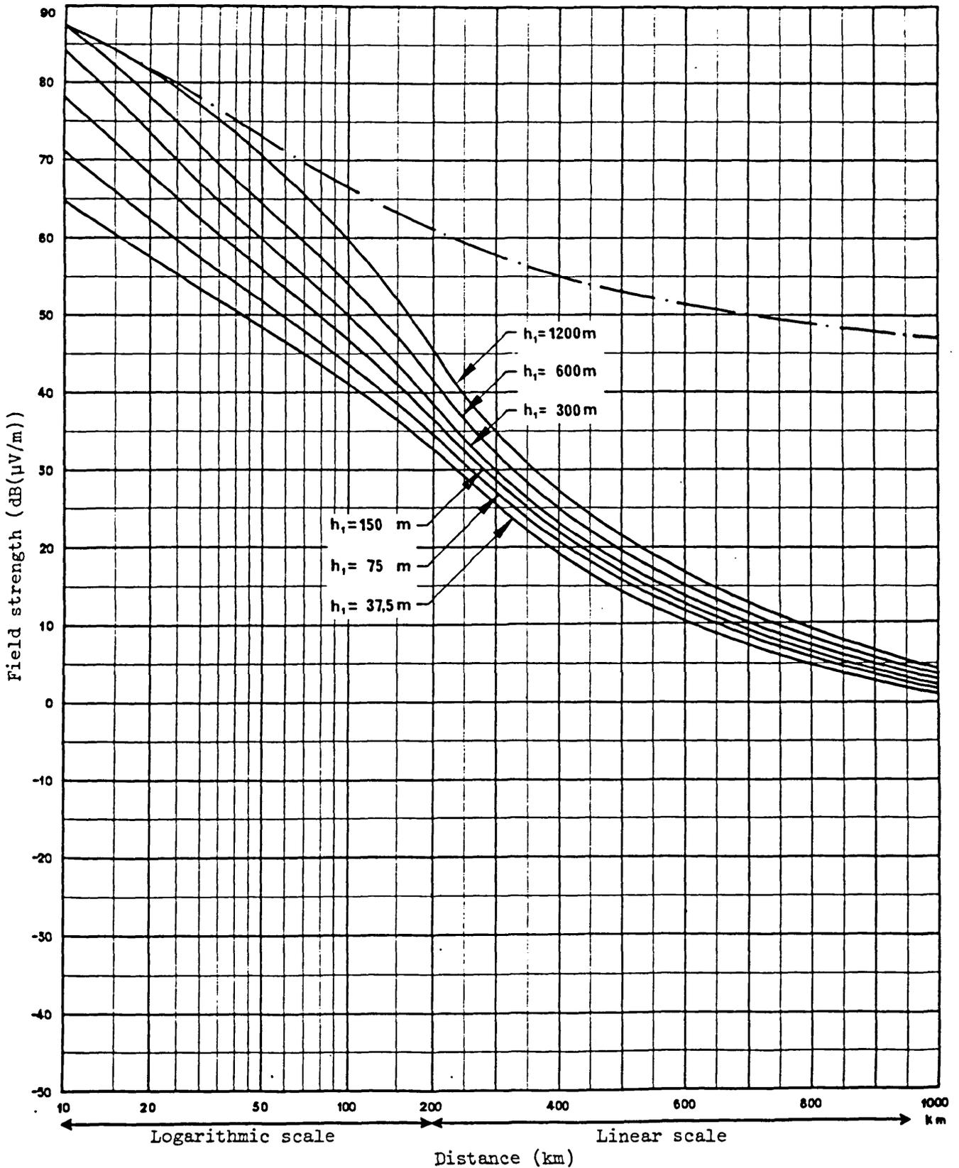
Figure 2.9 - Field strength (dB(μV/m)) for 1 kW e.r.p.
