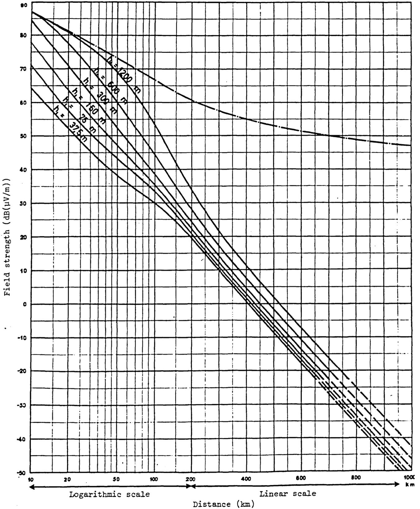
Figure 2.7 - Field strength (dB(µV/m)) for 1 kW e.r.p.
