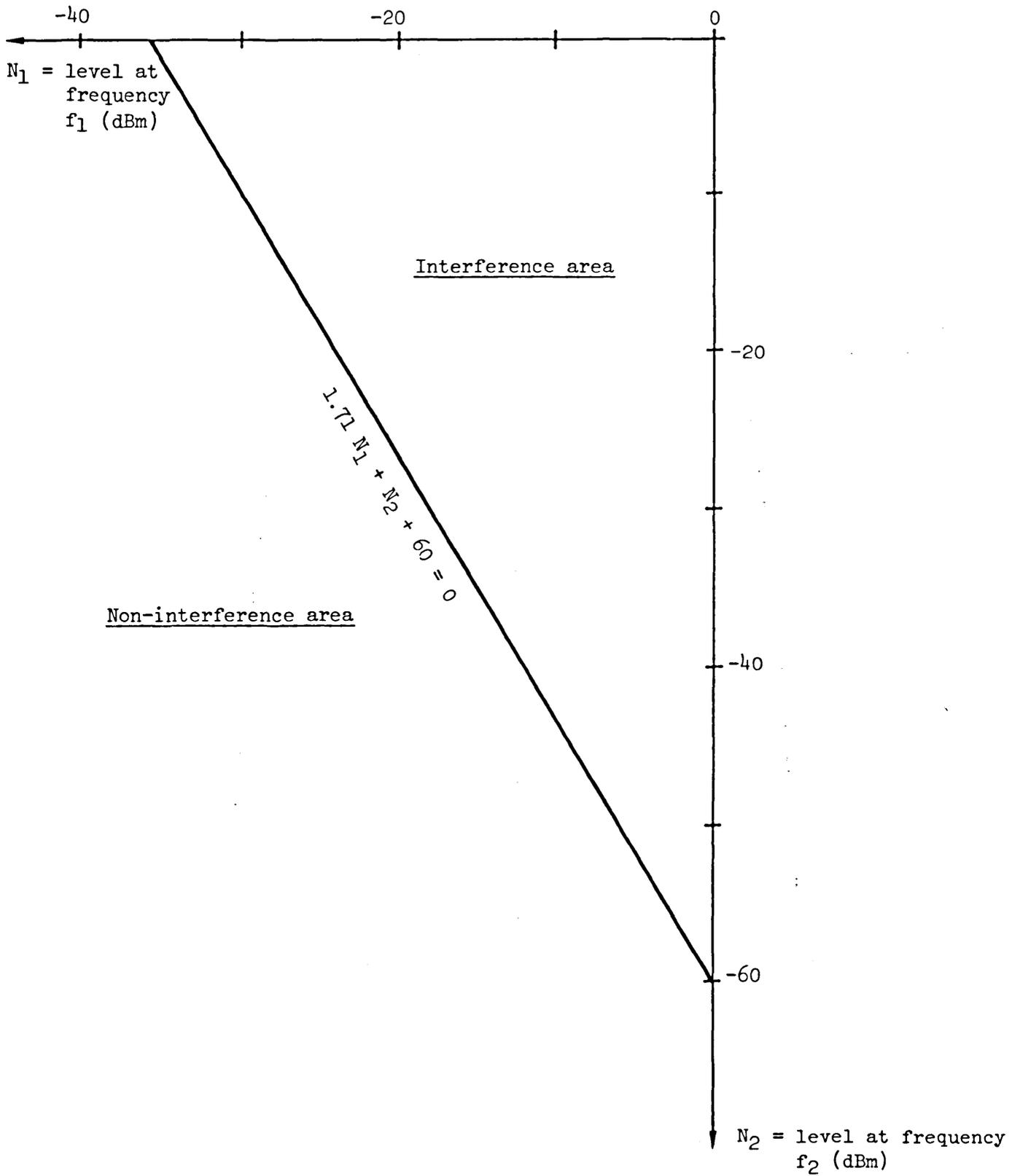
Figure 5.4 - Intermodulation threshold criterion
