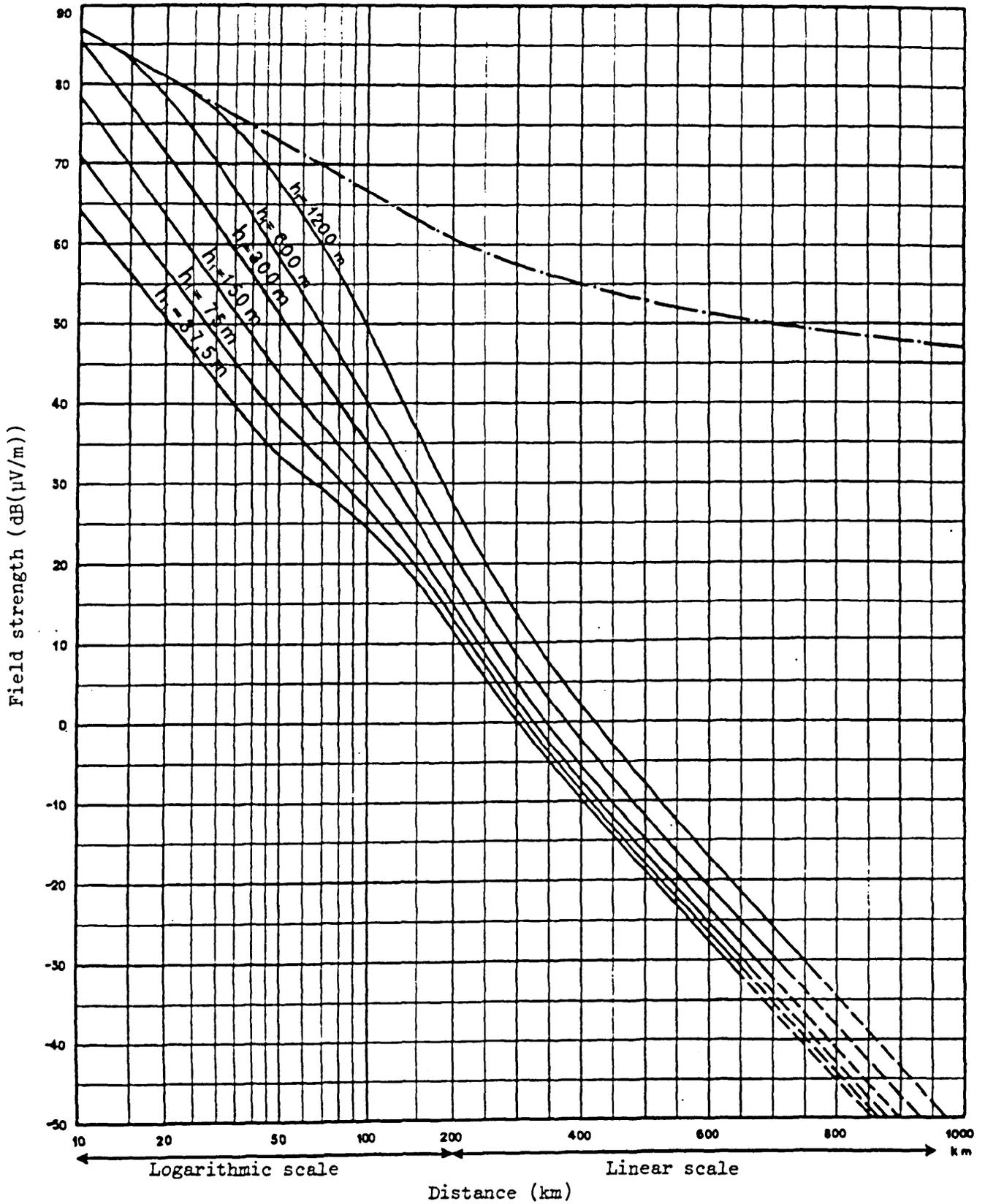
Figure 2.2 - Field strength (dB(μV/m)) for 1 kW e.r.p.
