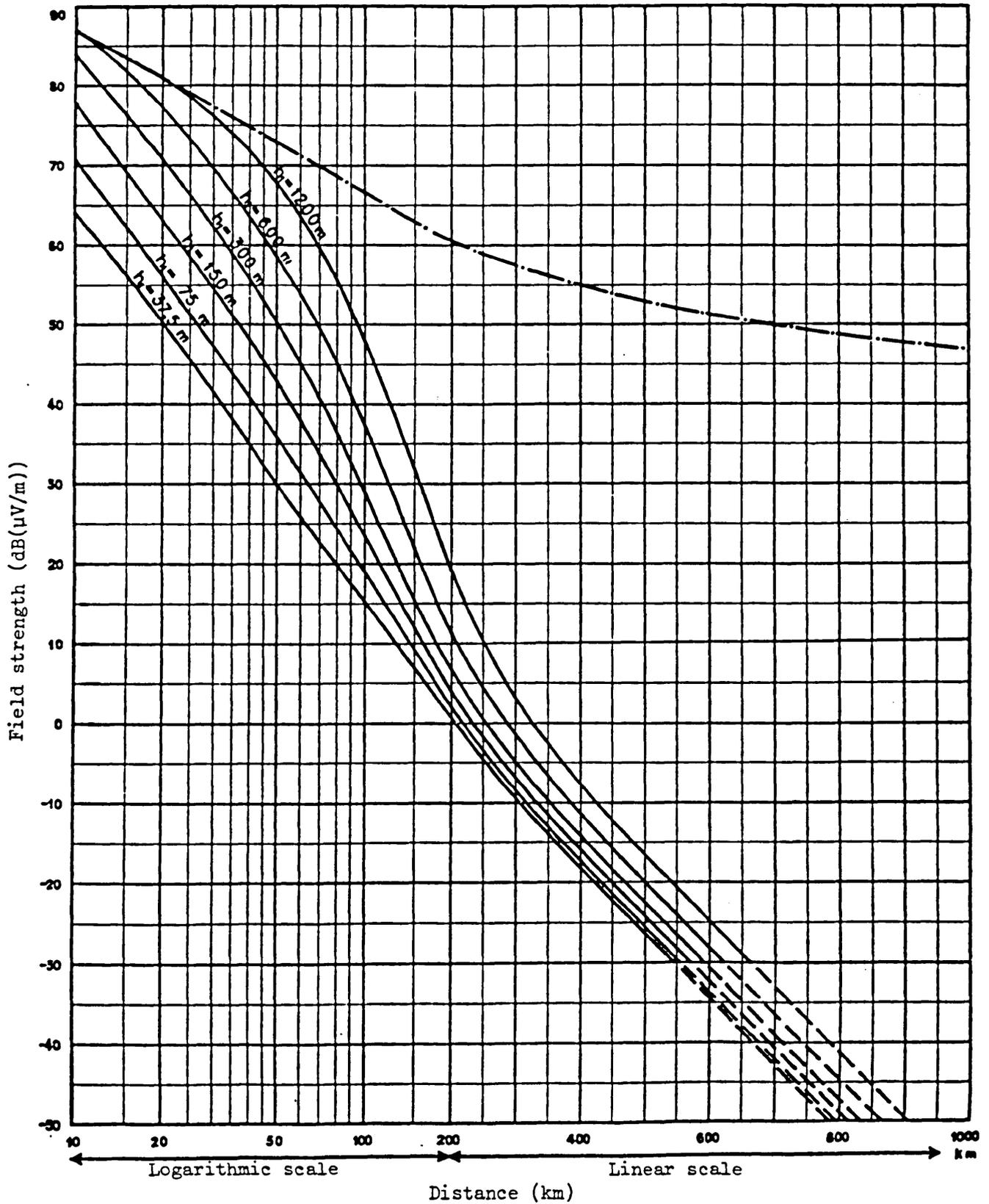
Figure 2.1 - Field strength (dB(μV/m)) for 1 kW e.r.p.
