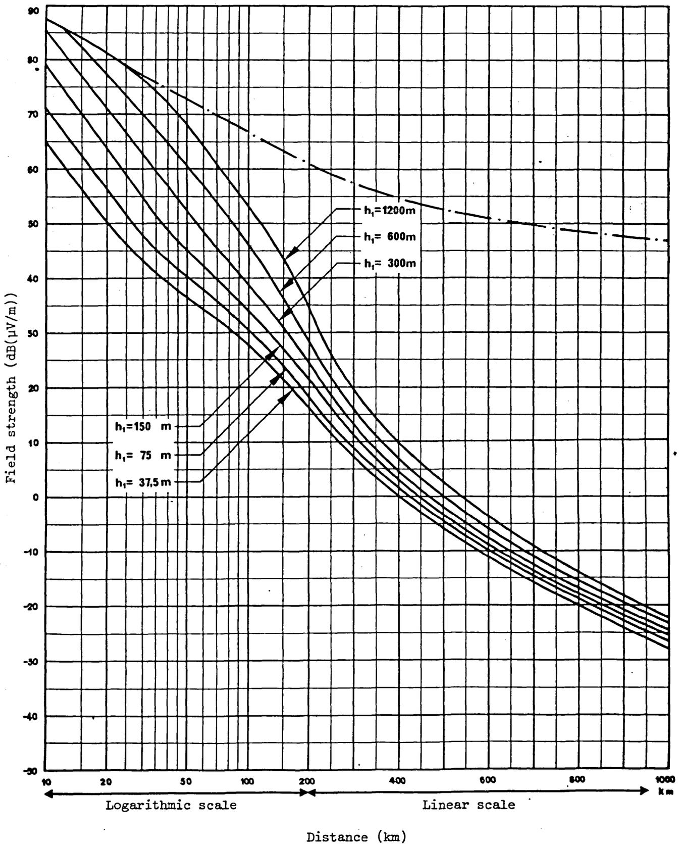
Figure 2.3 - Field strength (dB(µV/m)) for 1 kW e.r.p.
