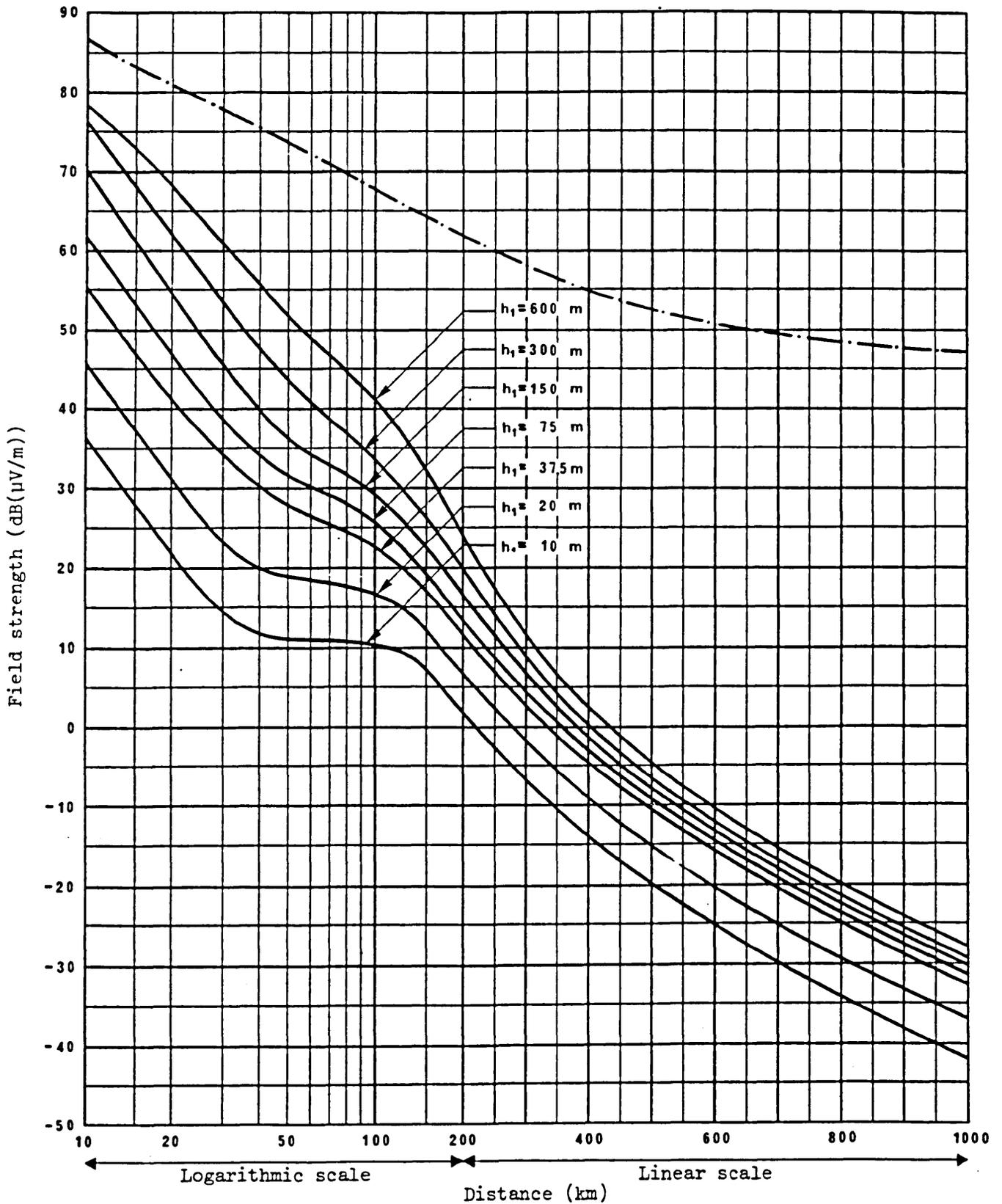
Figure 2.12 - Field strength (dB(µV/m)) for 1 kW e.r.p.
