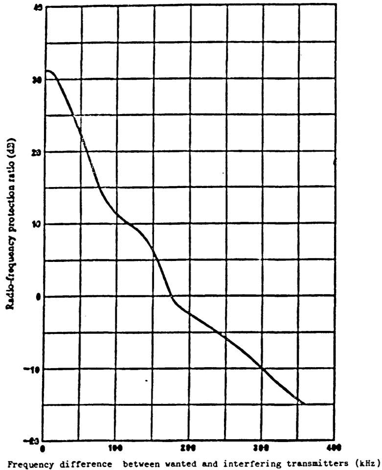
FIGURE 3.2 - Radio-frequency protection ratios for monophonic sound broadcasting in band 8 (VHF) using a maximum frequency deviation of  $\pm 50$  kHz
