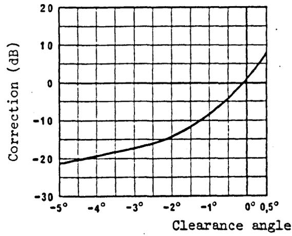
Figure 2.17 - Receiving terrain clearance angle correction (VHF)
