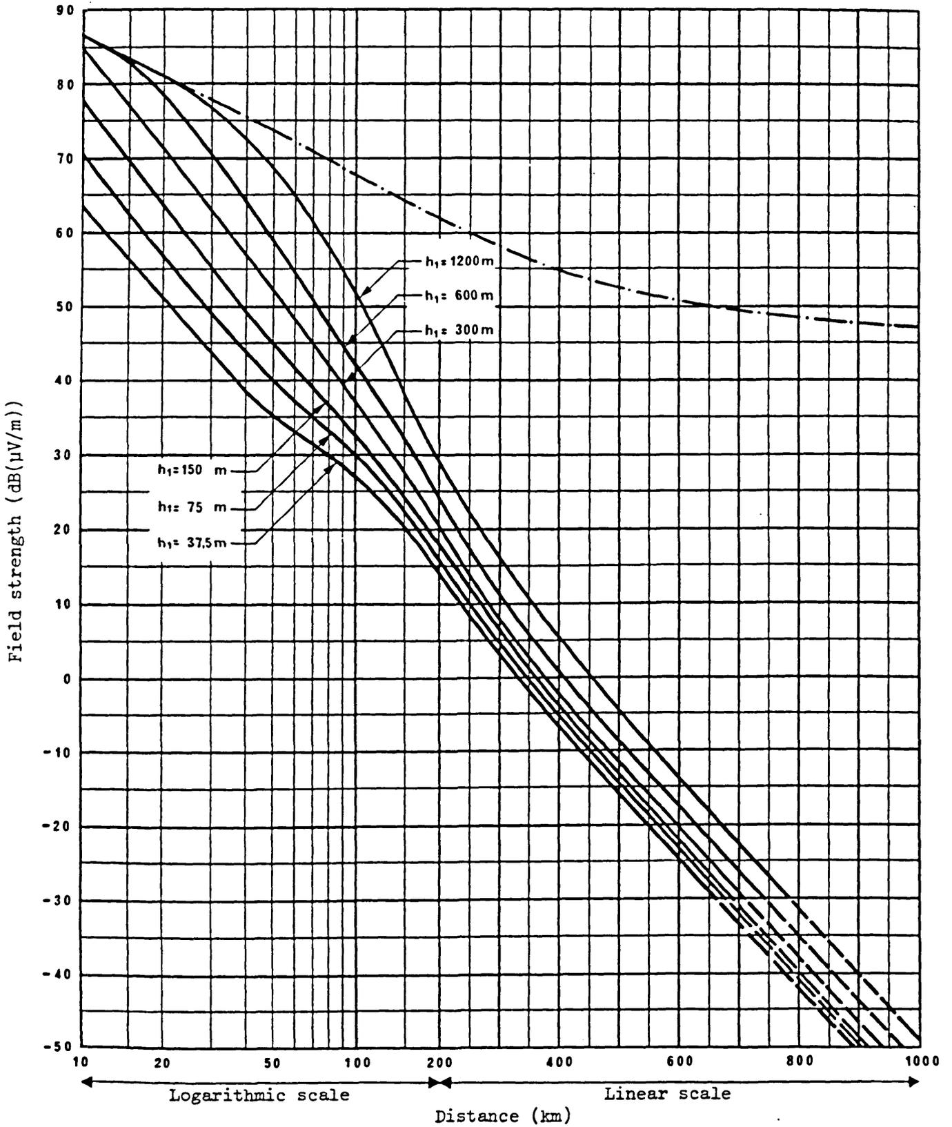
Figure 2.6 - Field strength (dB(μV/m)) for 1 kW e.r.p.
