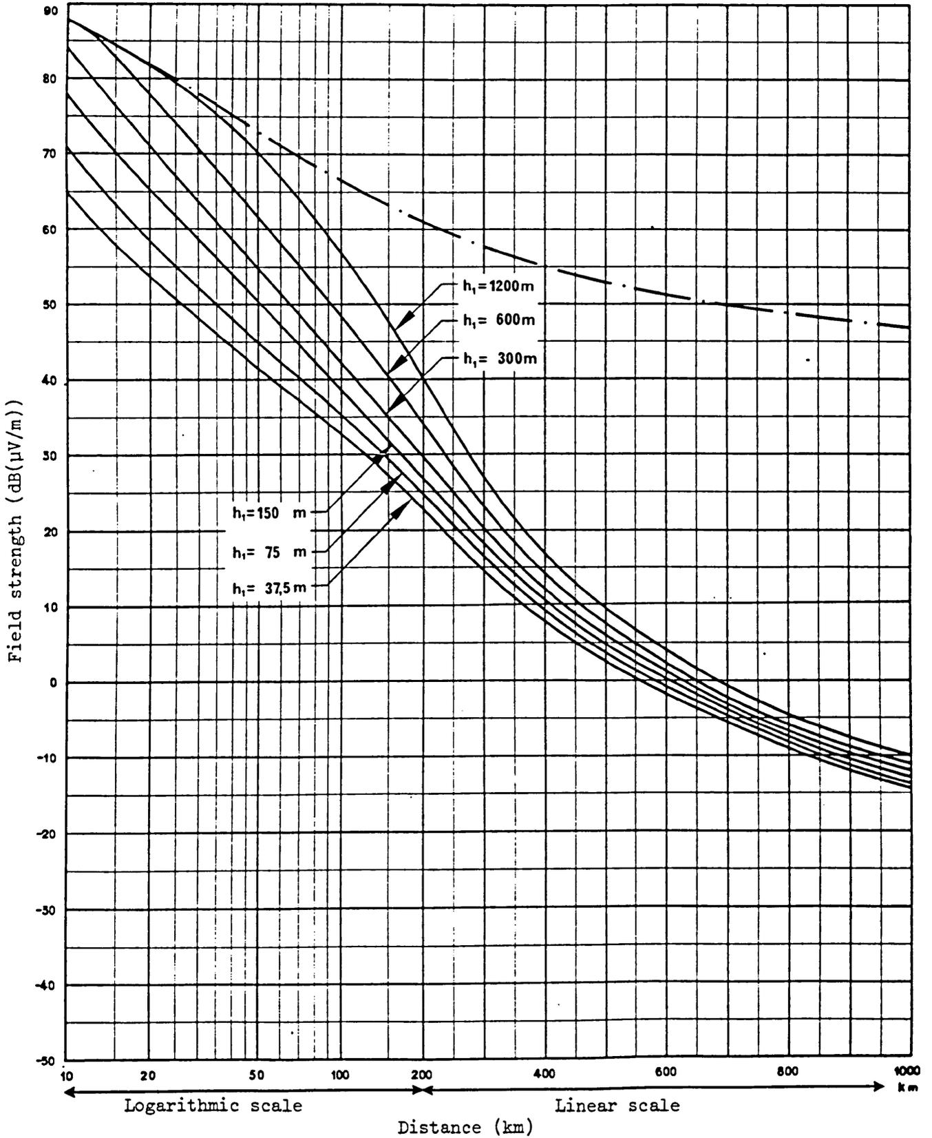
Figure 2.5 - Field strength (dB(µV/m)) for 1 kW e.r.p.
