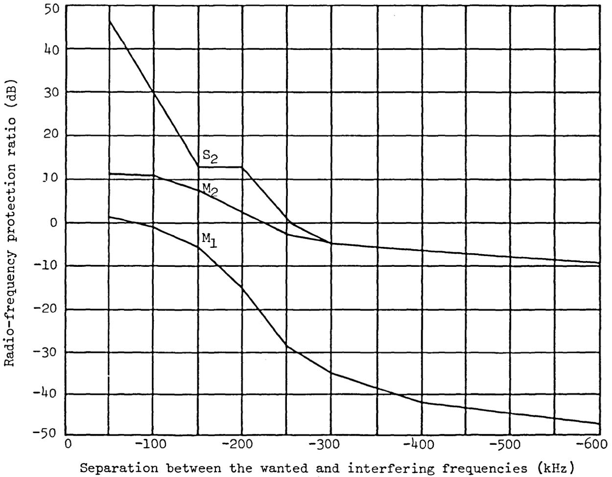
Figure 5.1 - RF protection ratios for a monophonic or stereophonic FM emission with interference by an FM or AM narrow-band emission. Steady interference. (Average curves for the ratios measured on domestic receivers.)
