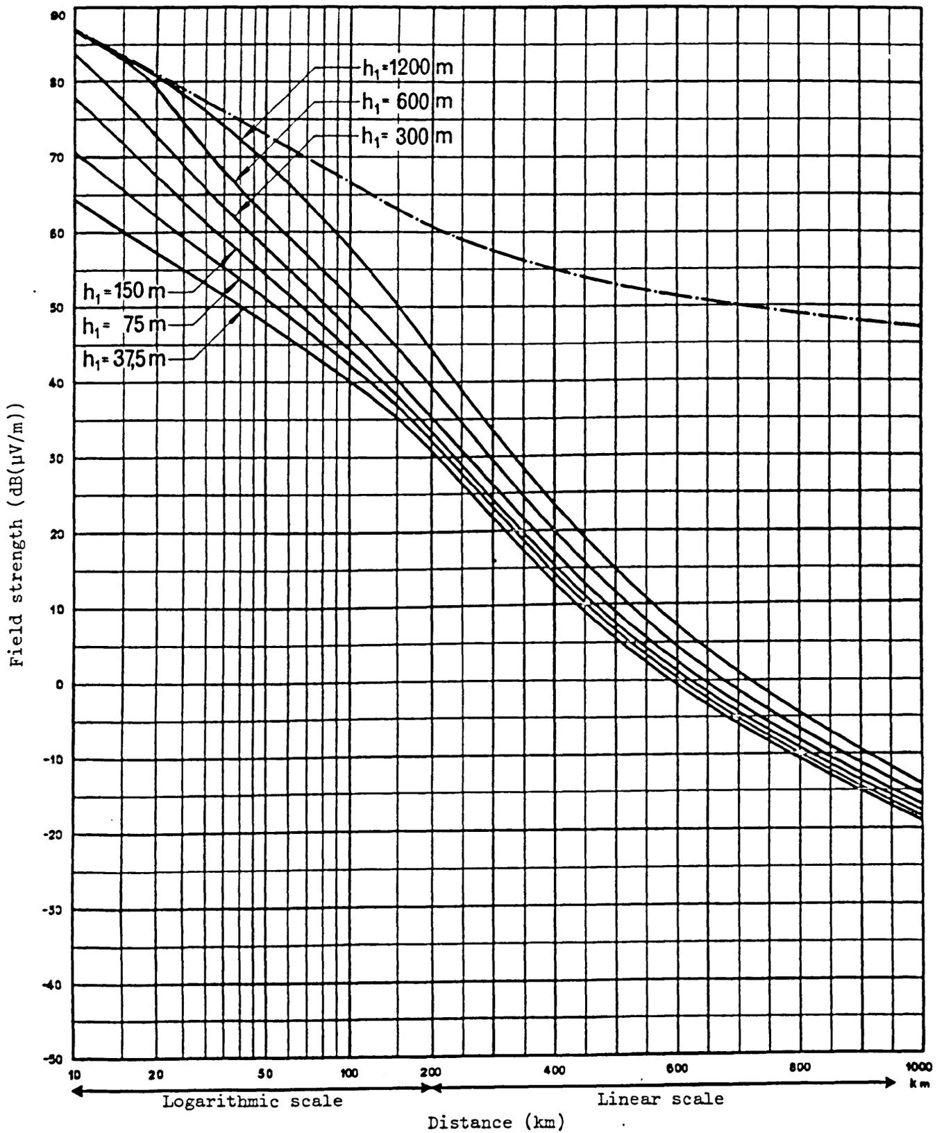
Figure 2.8 - Field strength (dB(µV/m)) for 1 kW e.r.p.
