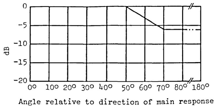
Figure 1 - Discrimination obtained by the use of a directional receiving antenna for the television stations in the band 87.5 to 100 MHz
