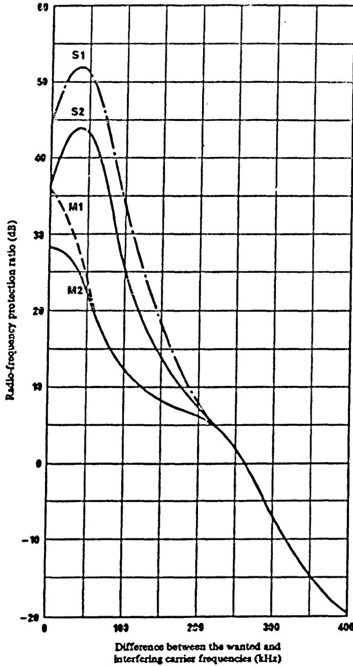
FIGURE 3.1 - Radio-frequency protection ratio required by broadcasting services in band 8 (VII-F) at frequencies between 87.5 MHz and 108 MHz using a maximum frequency deviation of  $\pm 75$  kHz
