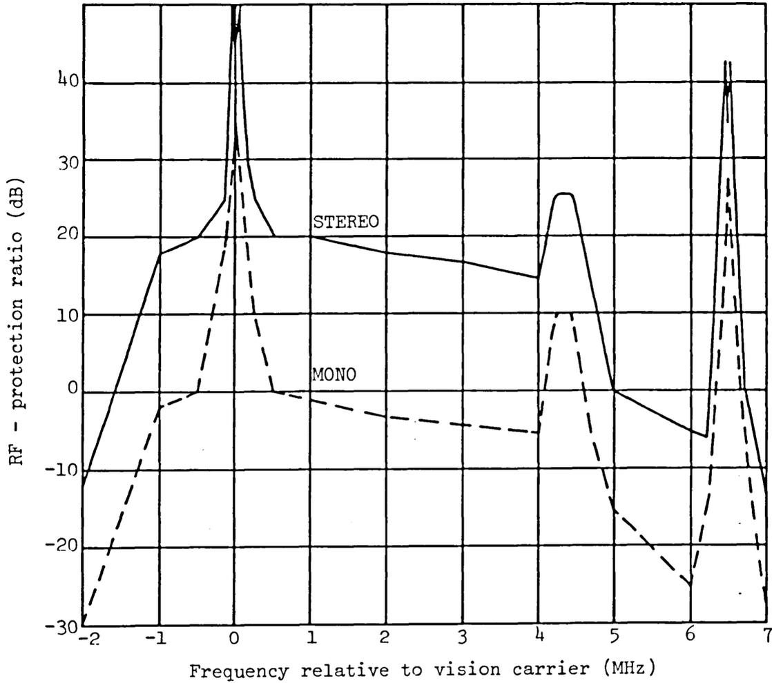
Figure 4.2 - Radio-frequency protection ratio required by FM sound broadcasting against interference from D/SECAM television transmissions in the band 87.5 to 100 MHz (steady interference)
