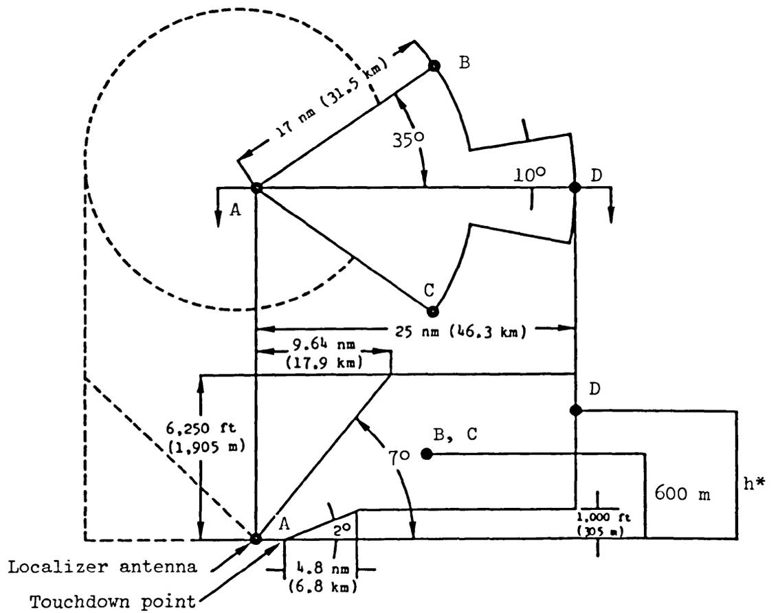
Note : The dash line shows the limits of ILS back beam protection volume which may have to be considered; in this case, the range and height are indicated.
