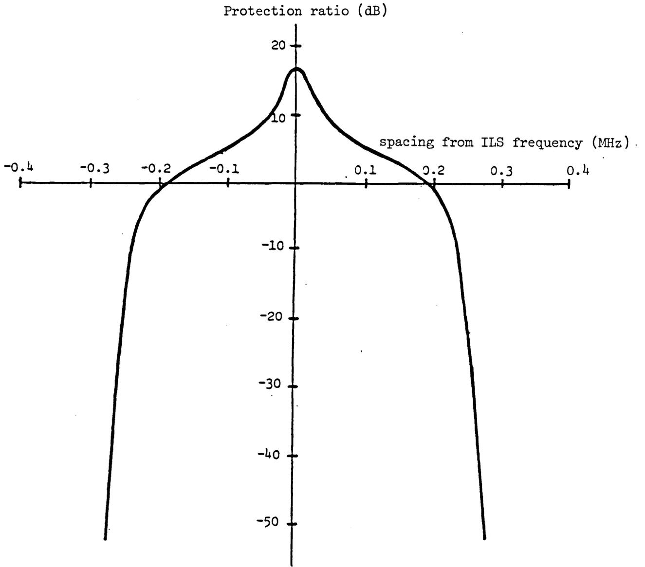
Figure 5.3 - Protection ratio for Type A 1) interference
