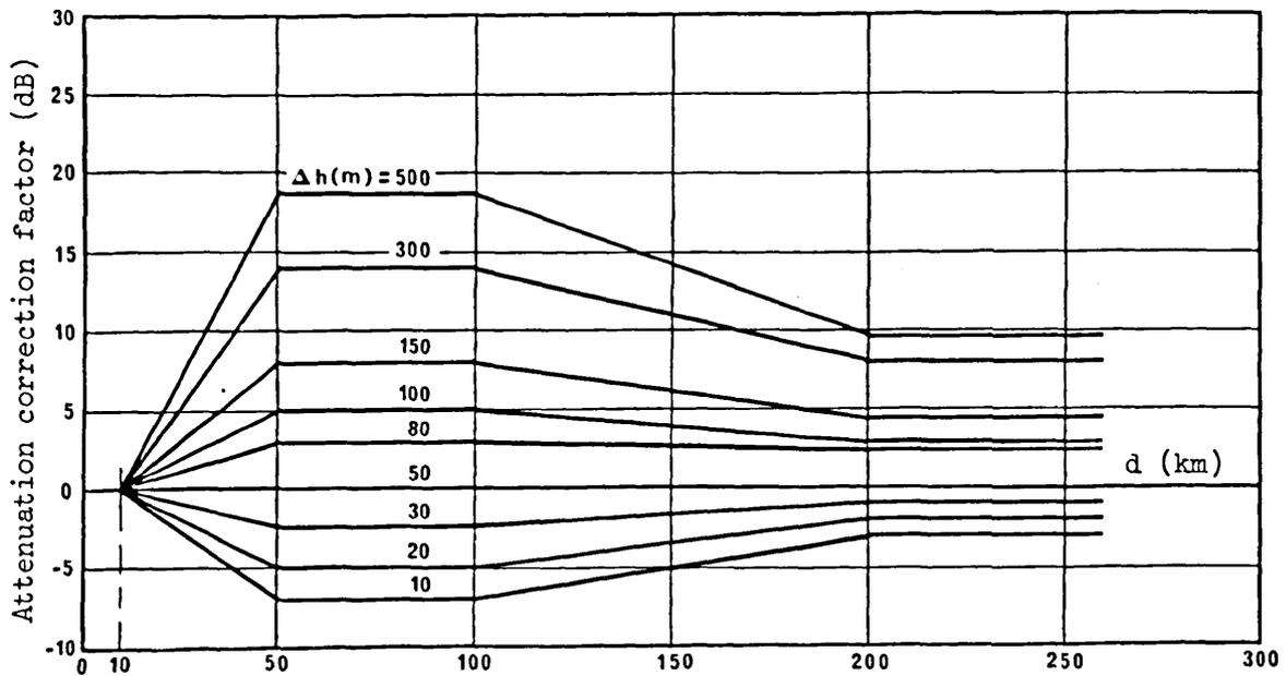
Figure 2.14 - Attenuation correction factor as a function of the distance from the transmitter for various values of Δh
