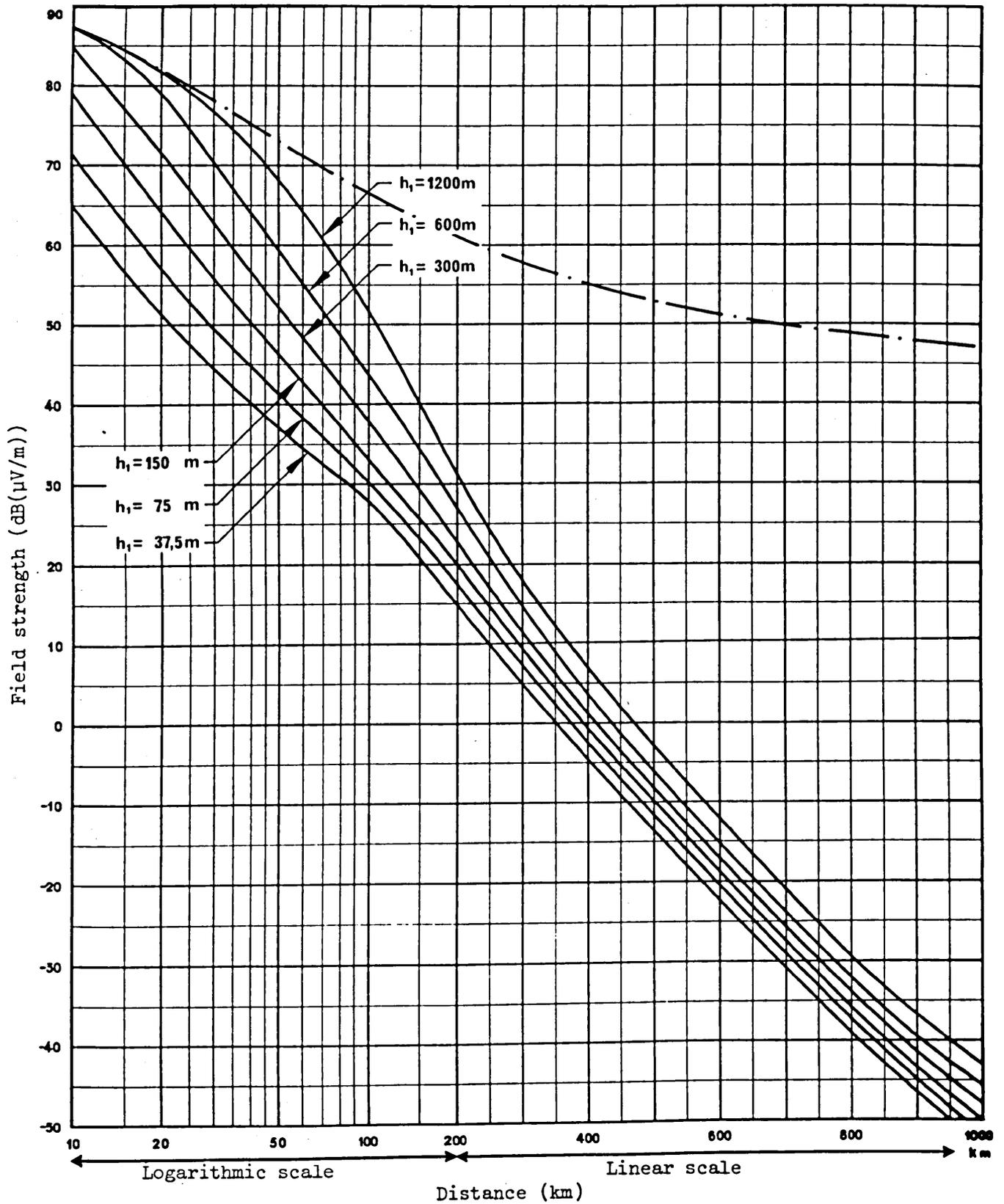
Figure 2.4 - Field strength (dB(µV/m)) for 1 kW e.r.p.
